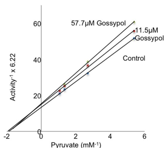
**Figure 3.** pH 8.00 Lineweaver-Burk plot, obtained as in the previous figures. Note that the lines intersect differently than in previous figures, indicating noncompetitive inhibition behavior.
