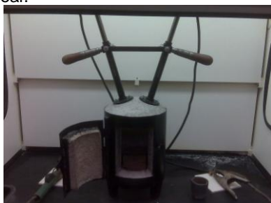
Figure 2. Furnace Constructed for My Research Sample Preparation
