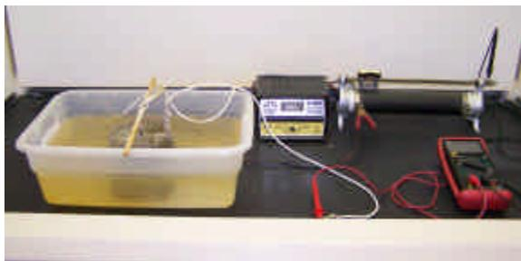
Figure 3. Electrolytic reduction set up. Battery charger provides DC power supply. Charger is wired to a variable resistor to control current and monitored by a volt/amp meter.
