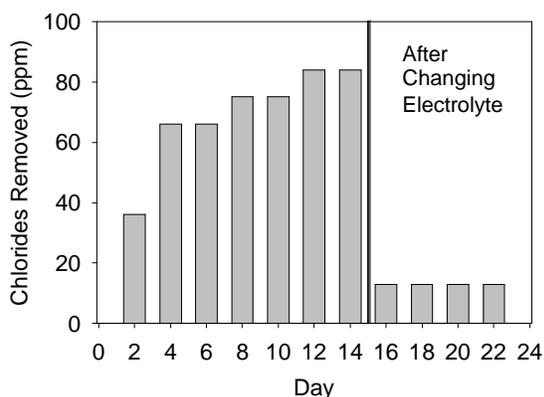
Figure 4. Chloride removal. Chlorides removed from the Brenham specimen measured in parts per million (ppm). Samples were tested every two days. After day 14, electrolyte was changed. Similar graphs were generated for each specimen.
