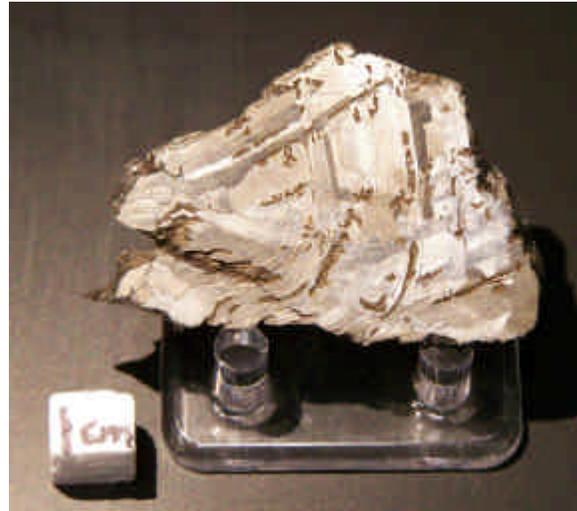
Figure 6. Nantan specimen after electrolytic reduction. Meteorite has been etched with nital to reveal the coarse Widmanstätten lines.
