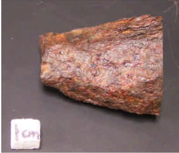
Figure 5a. Severely oxidized Brenham specimen. Specimen was surrounded with approximately 1 mm of oxidation.
