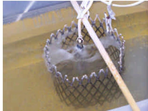
Figure 2. Close up of electrolytic reduction. A meteorite specimen is suspended in with only the Mueller clip of the cathode wire immersed in electrolyte. Note: Foam is normal and comes from H<sub>2</sub> and O<sub>2</sub> gas formed from the electrolysis of NaOH solution.
