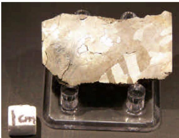
Figure 10. Campo del Cielo specimen. Meteorite has been etched with nitol and reveals the coarse Widmanstätten lines.
