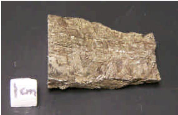
Figure 5b. Brenham specimen after electrolytic reduction. Notice oxidation has been removed in the process.
