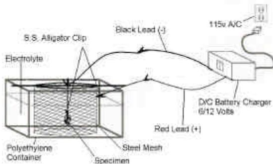
Figure1. Electrolytic reduction cleaning arrangement.
