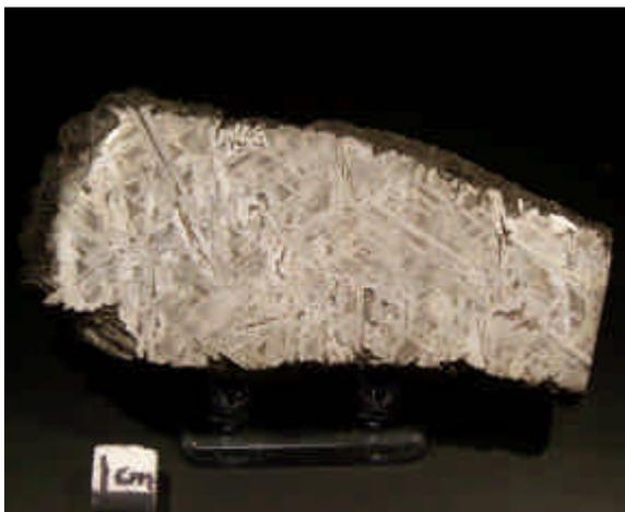
Figure 9. Elyria specimen after electrolytic reduction. Notice oxidation has been removed and no longer infiltrates between the Widmanstätten lines.
