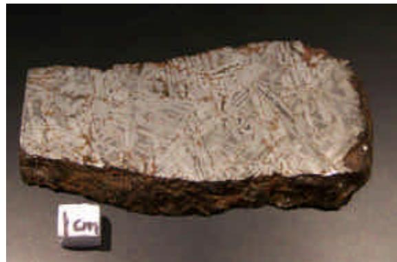
Figure 8. Oxidized Elyria specimen. Oxidation surrounds the edges of the meteorite and also infiltrates the Widmanstätten lines.
