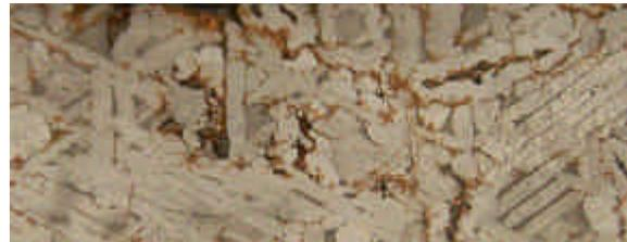
Figure 7. Close up of Elyria meteorite. Notice oxidation between Widmanstätten lines.
