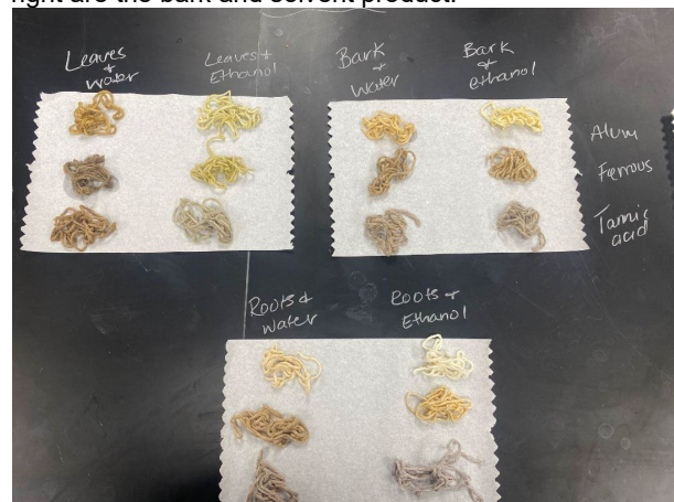
Figure 5. The dyes cotton yarn after washing and air drying. The top left is the leaves product, the top right is the bark product, and the bottom is the roots product.
